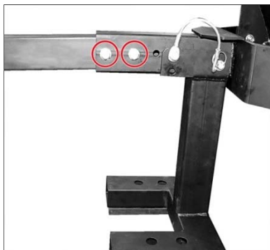
Mounting the drawbar with trailer coupling
